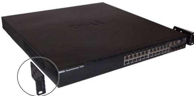
Figure 1-11. Fixation des supports
